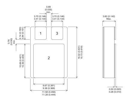
Bipolar NPN Device in a Hermetically sealed Ceramic Surface Mount Package for High Reliability Applications
